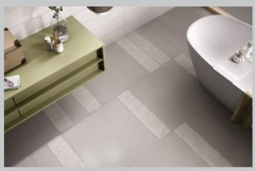
Installation: Manufacturer recommends on-set (stacked) pattern like the photo above. If a staggered pattern is preferred, tile should overlap no more than 20%. Use a high bond, property thin set. Tiles are non-rectified. Allow a min. 1/16″ grout joint. Use of leveling piece such as Tuscan Seamclip™.
